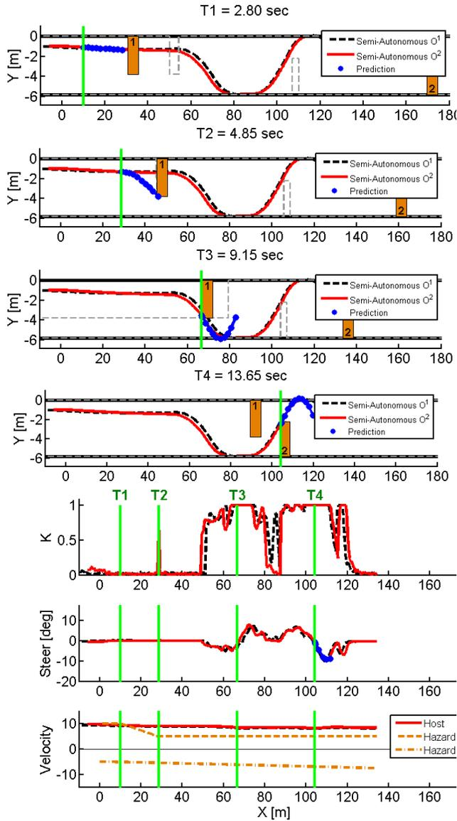
FIGURE 7. EXPERIMENTAL RESULTS OF SEMI-AUTONOMOUS CONTROLLERS NAVIGATING AMONG MOVING HAZARDS USING 1ST- AND 2ND-ORDER HAZARD POSITION PREDICTIONS
