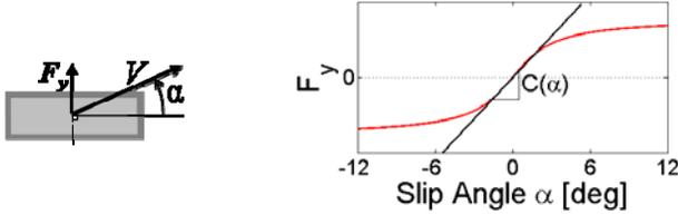
FIGURE 3. TIRE COMPLIANCE MODEL ILLUSTRATING VELOCITY  $V$ , SLIP ANGLE  $\alpha$ , AND LATERAL FORCE  $F_y$
