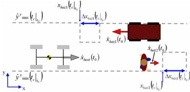
FIGURE 4. ILLUSTRATION OF CONSTRAINT PLACEMENT ( $Y_{MAX}^Y, Y_{MIN}^Y$ ) FOR MOVING HAZARDS
