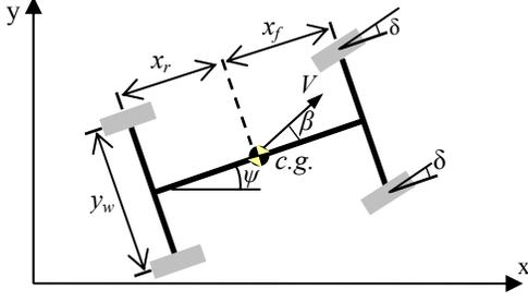
FIGURE 2. VEHICLE MODEL USED IN MPC CONTROLLER
