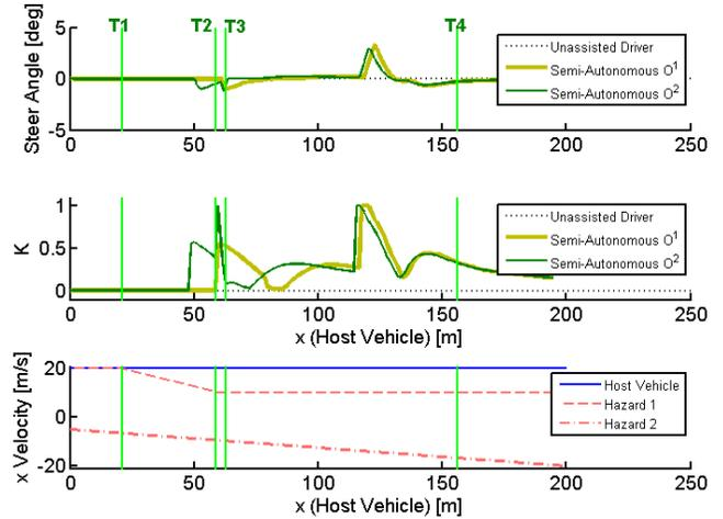
FIGURE 6. SIMULATION RESULTS COMPARING SEMI-AUTONOMOUS CONTROLLER PERFORMANCE AMONG MOVING HAZARDS USING A 1ST- AND 2ND-ORDER PREDICTIONS OF FUTURE HAZARD POSITION
