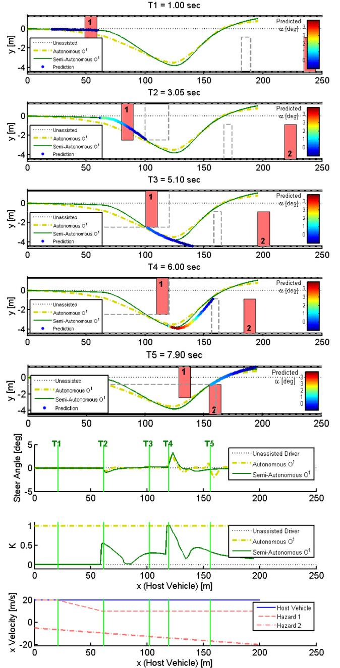
FIGURE 5. SIMULATION RESULTS COMPARING AUTONOMOUS AND SEMI-AUTONOMOUS CONTROLLER PERFORMANCE AMONG MOVING HAZARDS
